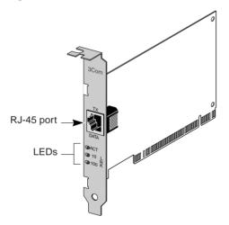
The OfficeConnect NIC backplate has three light-emitting diodes (LEDs):
